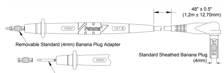
Standard .80" (2mm) Pin Tip Probe
